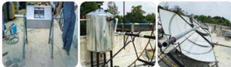
Fabricated Mobile Blancher unit for Turmeric processing and Steam Water Separator with Insulation Cover and CPC Panels
